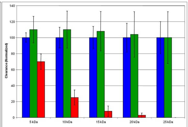
\*Typical results of patient dialyzers using the ClearFlux™ compared to polysulfone high-flux dialyzers using dextran molecular probes. Clearance data shows that the ClearFlux™ processed dialyzers are approximately equivalent to new dialyzers within experimental variances of the method.
