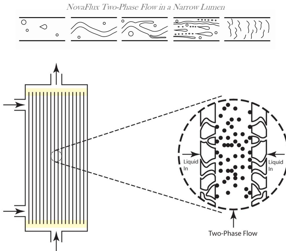
A schematic showing *in-situ* formation of the two-phase flow during dialyzer cleaning. The liquid flows from the dialysate side to the lumen side by backfiltration and is mixed with air to form the two-phase mixture in the fiber lumens. This process cleans the dialyzer membrane and headers at the same time.
